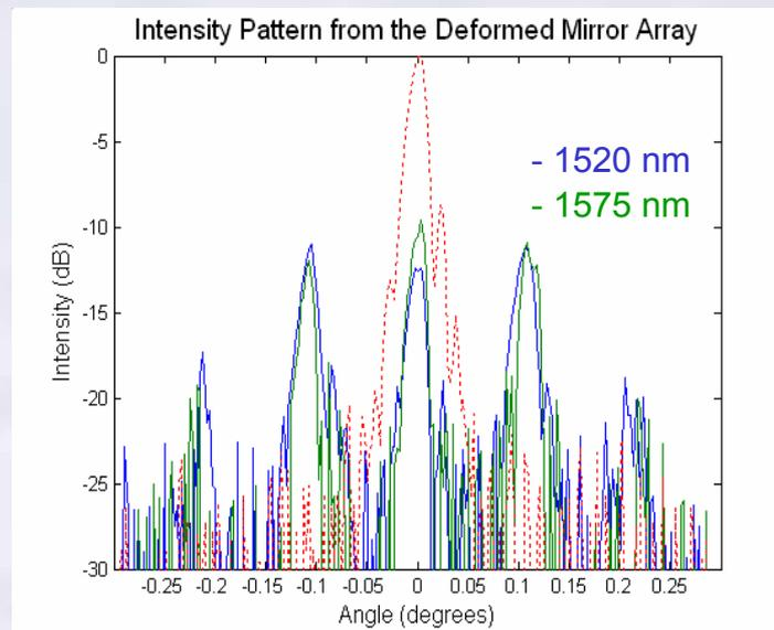
Experiment confirms broad wavelength spectrum operation
