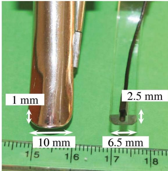
Fig. 7 Prototype blade compared to Miller 00 blade.
