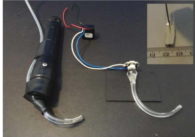
**Fig. 5** The full prototype is shown on the left and the LED, lens, and light guide assembly is shown on the right, with the tip shown with a ruler for scale (inset).
