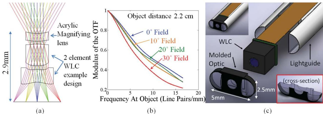
Fig. 9 (a) Raytrace diagram and (b) MTF for the modified WLC imager. (c) Shows the conceptual drawing of the entire laryngoscope tip, including the WLC, light pipe, and molded optic.
