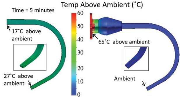
**Fig. 3** Temperature distribution model for tip-mounted and remote handle-mounted LED sources.
