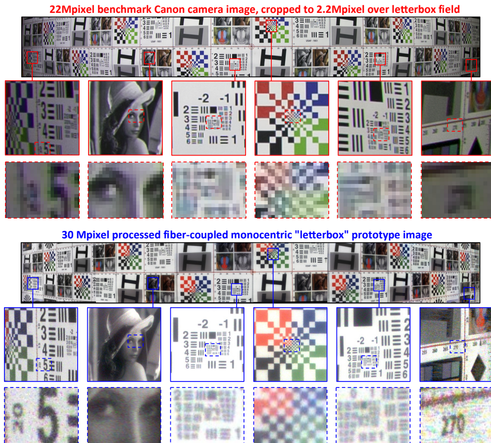
Fig. 12. Indoors comparison photos of the performance between Canon EOS 5D Mark II DSLR camera with Canon 8-15mm F/4 fisheye lens and the 2GS fiber-coupled F/1.0 monocentric prototype. Canon photo is cropped to match the prototype's letterbox 8:1 field of view.
