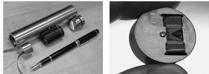
Fig. 3. (Left) Free-space WDM optomechanics, showing header, 50-mm focal length lens, and 600-lp/mm grating. (Right) Close-up of the device, electrical flex-circuit contacts, and I/O fiber ferrule on the cylindrical metal header.
