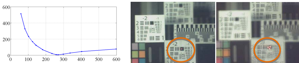
Figure 4. Range of measured distances (50-600cm) vs. radial separation of beam points measured in pixels on the y-axis along with example photographs that combine imaging with range finding (beam spots circled).
